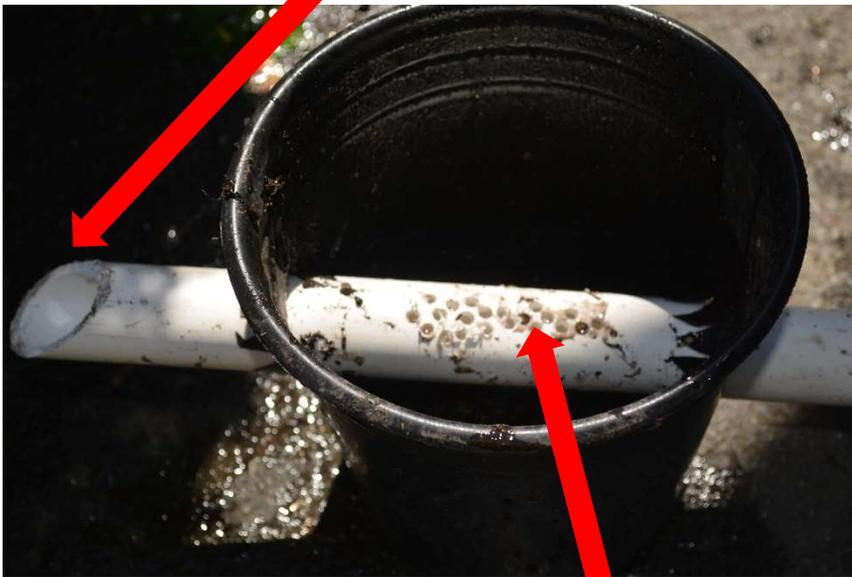
With a nail or drill, put a lot of large holes in one side of the pipe. With a hose, you can just cut a hole.
